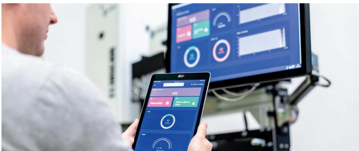
The CVS WEB module allows you to view vision system data without having to be present in front of the equipment.
