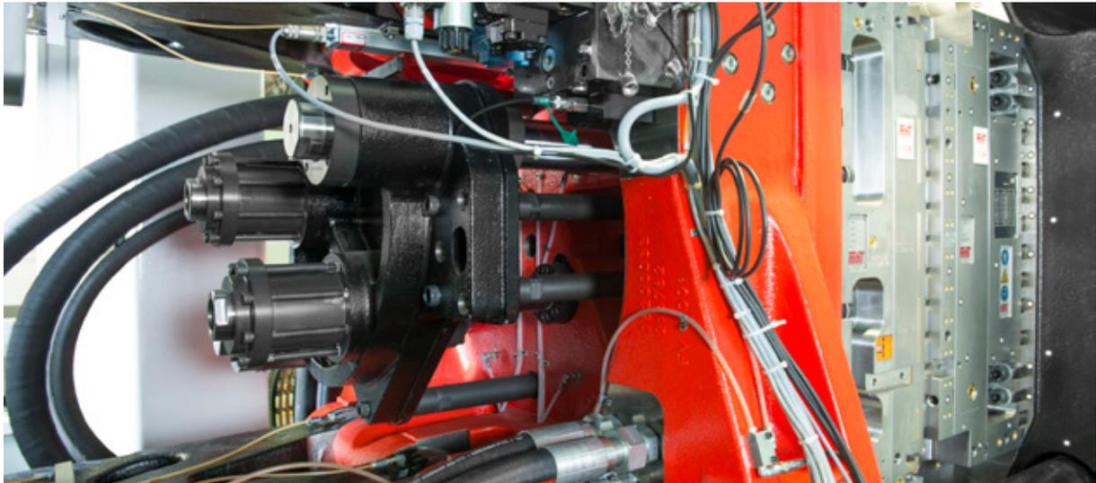
Clamping Unit – The toggle system and moving platen have been designed using FEM structural analysis. This optimizes mechanical inertia and ensures excellent resistance to mechanical stress. On the 220-ton machine the preform stripper plate is controlled by two hydraulic cylinders: one for preform release, the other for extraction.
