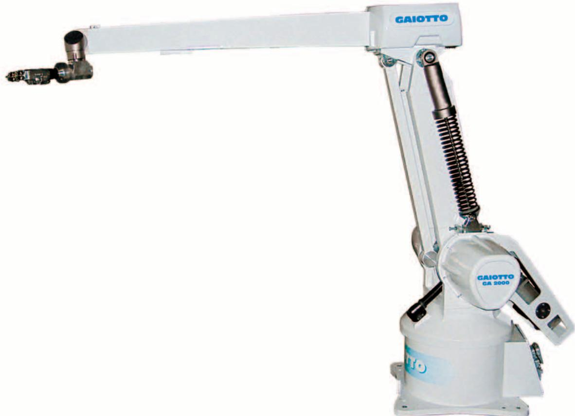
Hermetically sealed gearmotors, protective casings on all the motors and minimised number of connections all guaranteeing a suitable protection degree. Maintenance can be carried out in a user-friendly manner thanks to easy access to all moving parts. The electric control panel includes all the electronic control devices for the auxiliary axes and glaze flow rate control system (Mass Control system).
