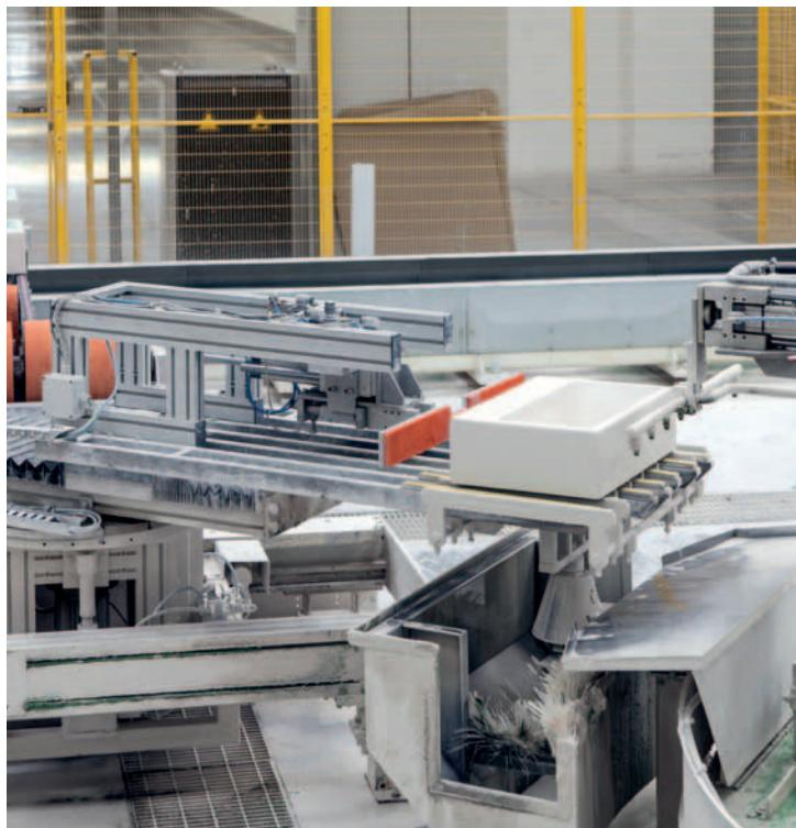
Conveyors are machines used to move workpieces from one location to the next - which may also be a few dozen metres away.
