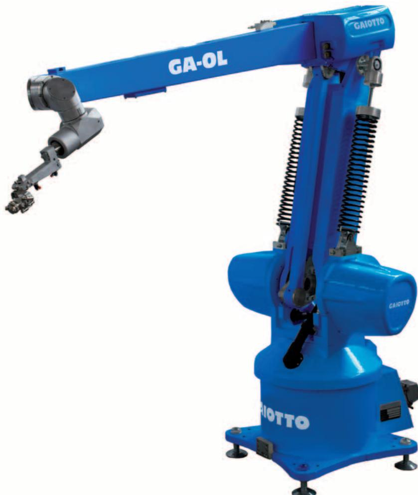
Hermetically sealed gearmotors, protective casings on all the motors and minimised number of connections all guaranteeing a suitable protection degree. Maintenance can be carried out in a user-friendly manner thanks to easy access to all moving parts. The electric control panel includes all the electronic control devices for the auxiliary axes and glaze flow rate control system (Mass Control system).
